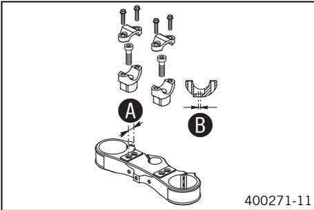
On the upper triple clamp, there are 2 holes at a distance **A** to each other.
