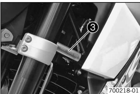
The Canada type label ❸ is on the right of the frame behind the steering head.
